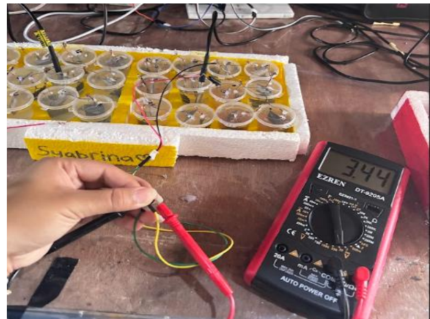
Figure 11. Voltage Generation Day 7 in Parallel MFCs
