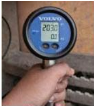
Figure 2. Hydraulic Pressure Measurement in Steering System
