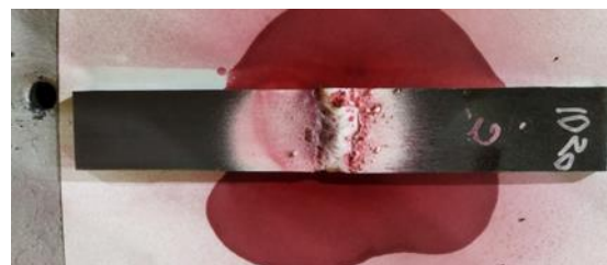
Figure 3. Results of red dye penetrant testing
