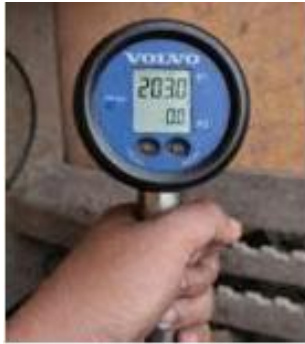
Figure 2. Hydraulic Pressure Measurement in Steering System
