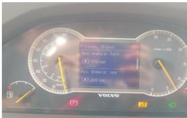
Figure 11. Actual Measurement Results on Monitor Unit
